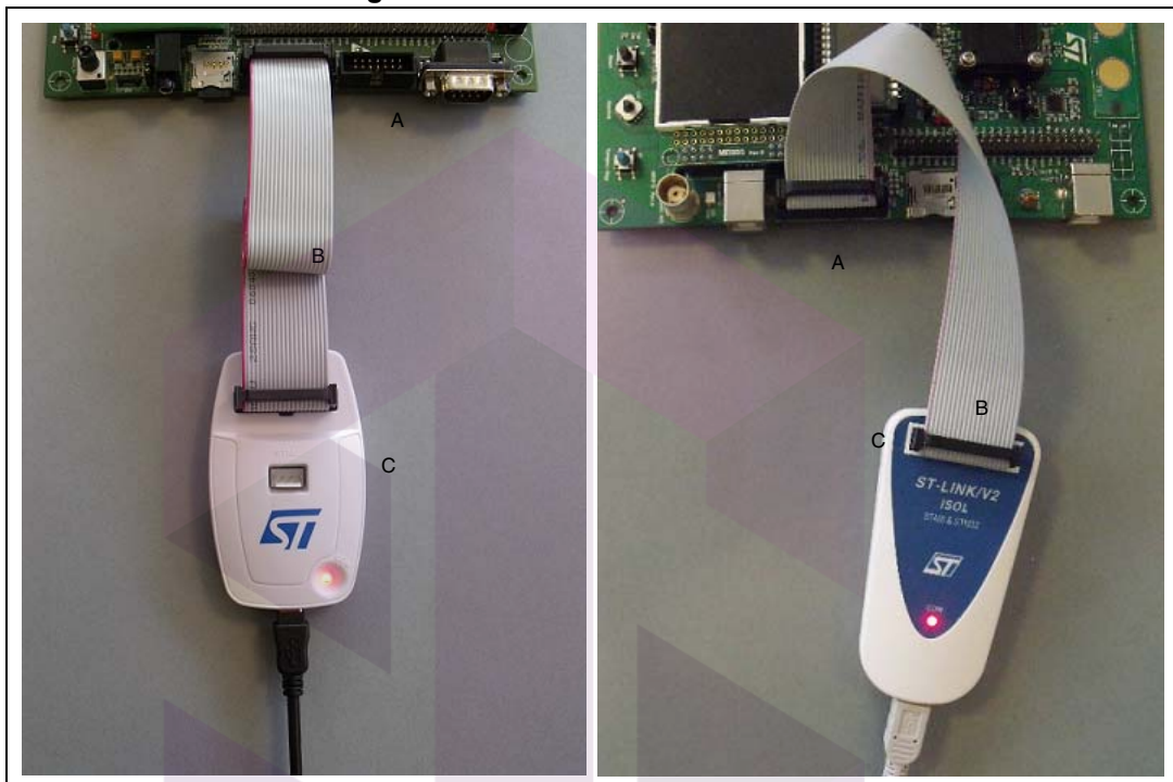
Figure 9. JTAG and SWD connection
